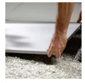
It can be installed onto gravel substrates simply by placing the slabs adjacent to one another or creating pathways by installing individual slabs onto the gravel support. It is also advantageous to integrate, below the layer of superficial gravel, another layer of gravel and or pebbles in order to ensure perfect drainage. This installation solution is functional, quick and with a strong visual impact.
